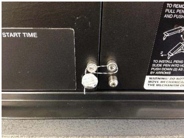
Open the door to the Chart Recorder. Locate the Wire Lockable Screws. Install the Regulatory Seal
