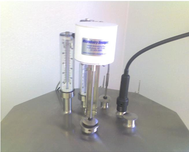
Agitator, Thermometers and Airspace Heater
