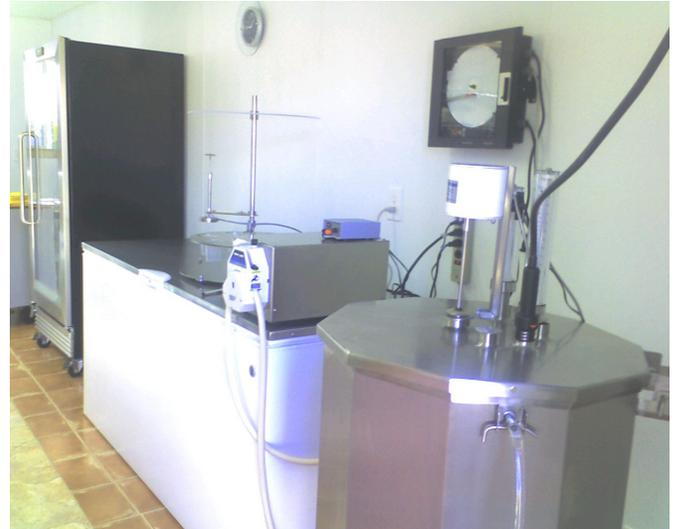
Typical Installation – Pasteurizer, Pump, Packager, Chiller
