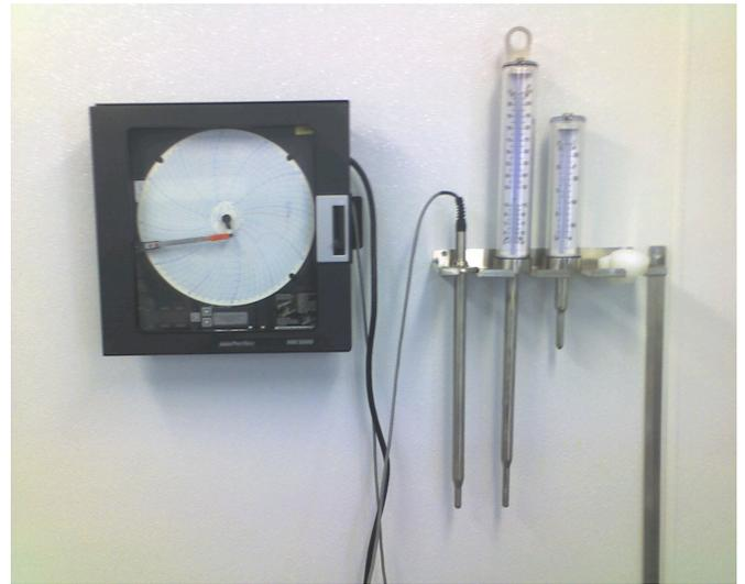
Chart recorder and probe, indicating thermometers
